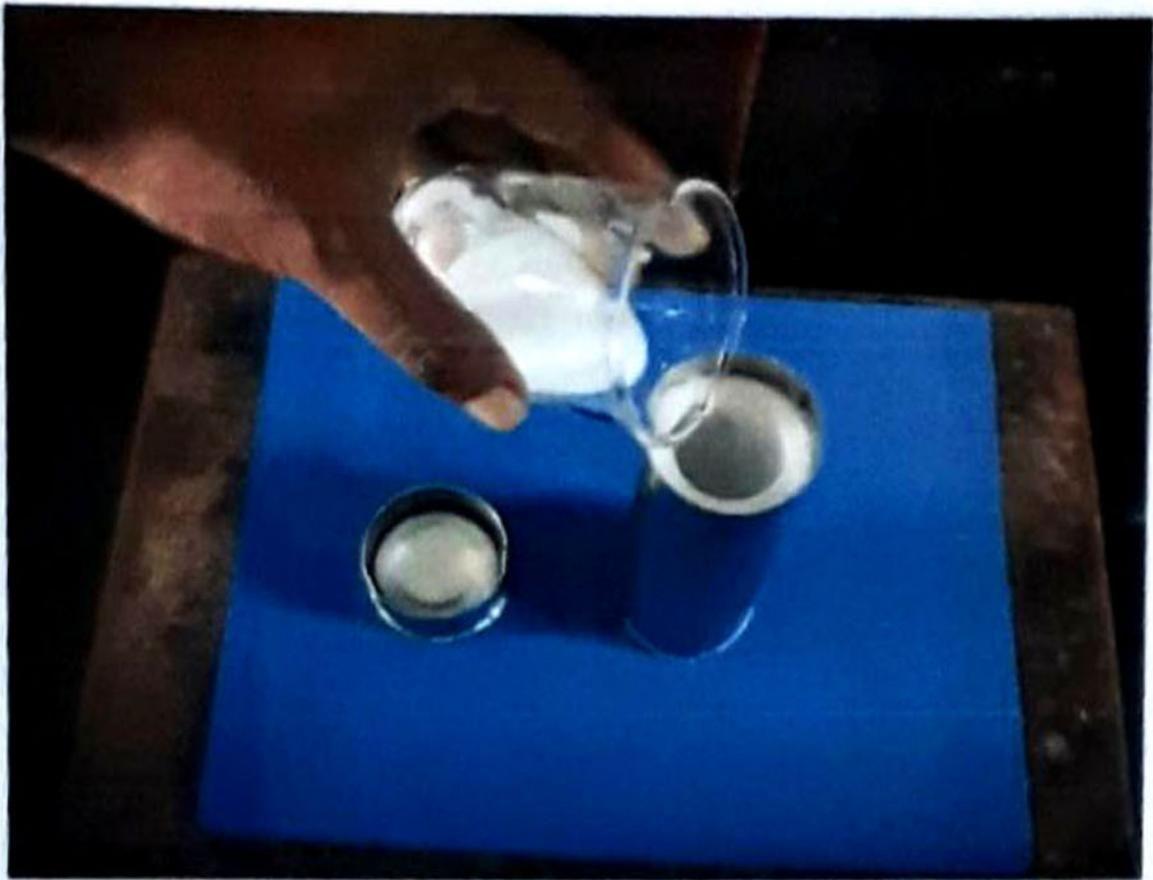
**Fig 2.2 (c) Pour Mix Solution into Stainless Steel Bomb**
