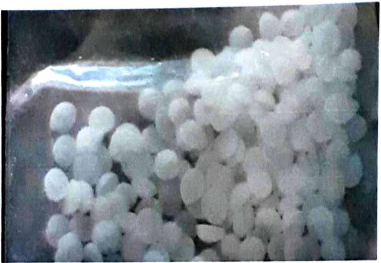
**Fig 2.1 (c) Potassium Hydroxide**
